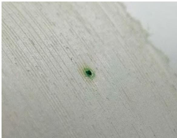
An extreme close-up of the burn mark at the first layer of insulation. Notice where the ionized copper left a green-colored mark.
