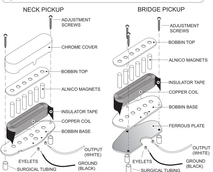
Exploded view of a single-coil **SweetSpot**™ **T-Series** replacement pickups for Telecaster®-style guitars.
